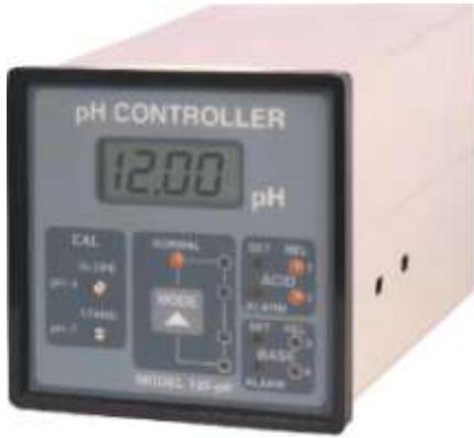
Model 100pH Controller is a panel mounted DIN size instrument with 3½ Digit LCD. Indicates pH when attached to a pH electrode. The membrane key pad Mode Switch in front allows indication of normal pH, Limits for Acid/Base together with additional alarm limits for Acid/Base. In addition, a Consent contact output is provided to be used in conjunction with an ORP Controller for ORP dosage.
